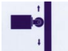
Optional guide rails and guide wheels to make the platform more stable
